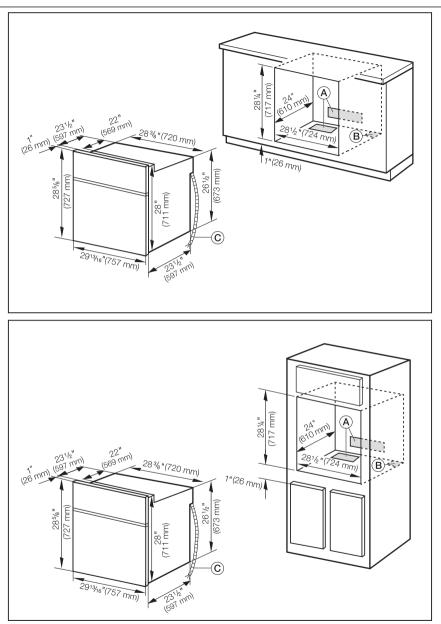
(a) Vent cut-out (min. 24"  $^2$  / 150 cm²) possible at rear **or** platform of cabinet (B) Cut-out for power cord (min. 1"  $^2$  / 3 cm²)
