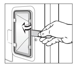
Slide the light cover out of the two clamps secured to the metal frame.
