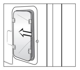
Press the light cover into the metal frame.
