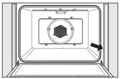
The silver data plate is located along the front side of the lower oven with the door open.
