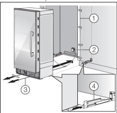
■ To protect the corners of the installation space, attach the supplied edge protector ① on both sides with adhesive tape.
