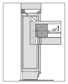
If the anti-tip brackets cannot be attached securely, an alternative anti-tip device can be used. Ensure that there is no "give" between the appliance and the anti-tip device.
