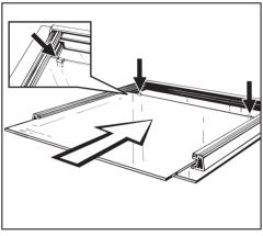
Slide the middle pane in slightly and then refit the seal. Then push the pane right in.
