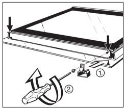
■ Refit the guides and screw the trim firmly back in position.
