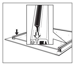
■ Fit the side seals for the inner panel in the grooves provided.
