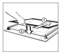
■ Fit the middle pane with the matt printed surface facing downwards. Make sure that the side seals do not slip and push the pane in as far as it will go.
