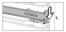
■ Push down on the tab at the front of the FlexiClip runner (1.).
