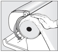
■ Turn the roller by hand in the direction you iron (see arrow) until the cover retaining slot is at the bottom.
