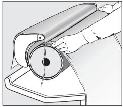
■ Insert the raw edge of the new ironing cloth into the retaining slot with the wrong side down. Keep side ties hanging free and smooth out.
