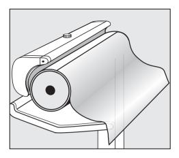
■ Completely unwind the cotton undercloth attached to the roller and let it hang down smoothly.
