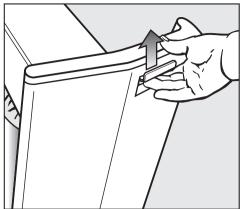
Hold the ironing table securely and pull on the release catch situated at the back of the ironing table on the right hand side.
