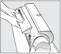
■ First remove the feed-in table by lifting it out of the right hand holder, then pull it out to the left of the roller.
