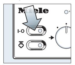
The **I-0** "On-Off" switch is used for switching the ironer on and off.
