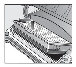
Replace with a new filter, and push it down into place.
