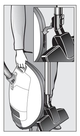
Warning: Always disconnect the vacuum cleaner from the electrical supply for maintenance work and for cleaning. Switch off at the wall socket and unplug it.
