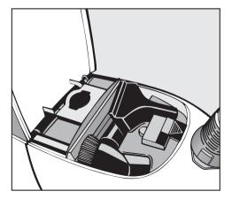
The different tools can either be fitted to the hand-piece or, as required, to the suction tube.
