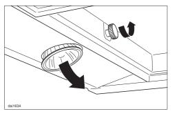
Turn the nut anti-clockwise as far as it will go. The halogen lamp will then drop down towards you.
