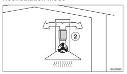
The silencer needs to be positioned between the exhaust socket and the directional unit ②. Ensure there is adequate space for fitting it.
