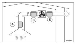
To minimise noise from the motor in the kitchen, the silencer should be positioned in front of the external motor ③ if possible, or, if the ducting is long, above the exhaust socket on the cooker hood ④. In the case of an external motor located inside the house, fitting a silencer behind the external motor ⑤ reduces the noise of the motor outside the house.
