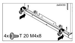
Secure the hood with the screws supplied.
