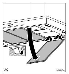
■ Remove the grease filters from the hood.
