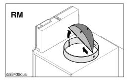
With vented mode (AE) insert the non-return flap in the exhaust socket if your ducting system is not equipped with one.
