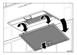
■ To remove a grease filter, release the locking clip. Then, open the filter to a 45° angle, unhook it, and remove it from the hood.
