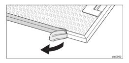
Before using the appliance remove the grease filter and remove the protective foil from the filter frame. Return the filter.
