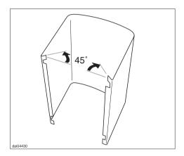
Bend the top hanging tabs 45° inwards. This will make installing the chimney extension easier. Be careful of sharp edges.
