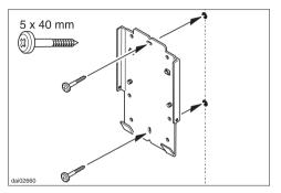
Lightly secure retaining plate A into position using 5 x 40 mm screws through the two holes and use the notches to align with the center line.
