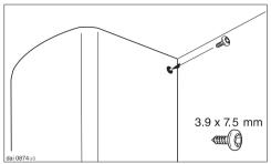
Secure the chimney extension to the upper retaining plate with two 3.9 x 7.5 mm screws.
