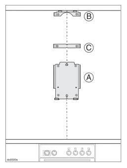
The ventilation system will be mounted to the wall through the use of retaining plates. Plate A is installed first, followed by plate B. Plate C should ony be used if the distance between plate A and plate B is greater than  $14 \frac{3}{8}$  " (365 mm).
