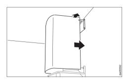
Pull the chimney extension slightly outwards and snap over the upper retaining plate B.
