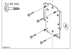
Screw four 5 x 40 mm screws into the upper and lower set of holes to secure retaing plate A.
