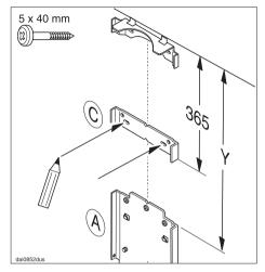
Retaining plate C should only be used if dimension Y is greater than  $14 \frac{3}{8}$ " (365 mm). It provides additional stability for the chimney extension.
