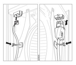
Plug the connectors on the canopy into the corresponding receptacles left and right of the motor assembly.
