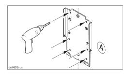
Drill 6 more <sup>1</sup>/<sub>8</sub>" (3 mm) holes through the now fitted retaining plate.
