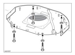
■ Secure the mounting plate to the ceiling using the 8 x 60 lag bolts. Once tight, make sure that the mounting plate can safely support the weight of the hood.
