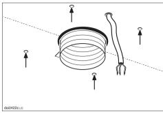
■ Drill four <sup>3</sup>/<sub>16</sub>" (5 mm) holes in the ceiling.
