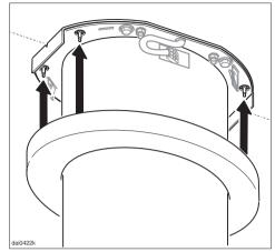
■ Finally, being careful not to scratch the chimney, push the cover plate up and onto its locking pins until it clicks into place. If installed correctly, the cover should be secure and flush against the ceiling.
