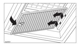
■ To remove the grease filter pull the locking clip forward. Lower the filter 45° unhook it at the rear and take it out. Support the grease filter so that it does not fall onto the cooktop.
