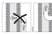
If the exhaust is ducted into an inactive flue, the air must be expelled parallel to the flow direction of the flue.
