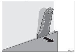
■ After removing the two screws from the chimney, slide the lever between the chimney and the chimney extension and gently apply pressure to ease the chimney from its hooks.
