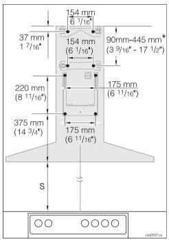
To prepare a backing plate, the spacings for the 5 mm screws need to be drilled as shown.
