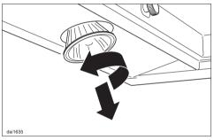
Turn the bulb counterclockwise and pull it out of its socket.
