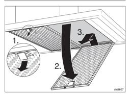
■ To remove the grease filters pull the locking clips, 1, forward. Lower the filter 45°, 2, unhook it at the rear, 3, and take it out. Support the grease filter so that it does not fall onto the cooktop.
