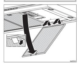
■ To remove the grease filter pull the locking clip forward, lower the filter down 45°, unhook it at the rear, and take it out.
