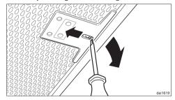
If the filters are incorrectly installed, insert a small screwdriver into the slit along its edge to disengage it from the casing.
