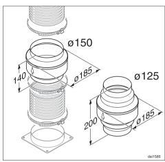
Besides appropriate insulation of the exhaust ducting, we recommend installing a condensate trap to collect and evaporate any condensation which may develop. This is available for ducts Ø 5" (125 mm) or Ø 6" (150 mm).
