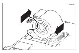
Plug the connection cable from the ventilation system into the blower motor.
