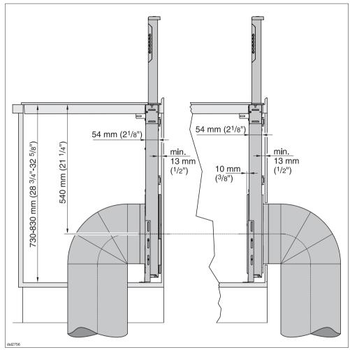
Exhaust air ducting to the front.
