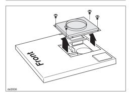
Remove the connection plate from the front of the appliance.
