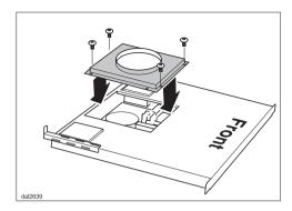
The connection plate is installed the same way as described for the blower box.
