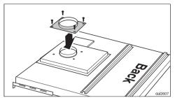
Mount the vent collar on the rear of the ventilation system.
