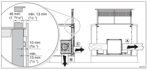
Exhaust air ducting using the DAG 500 internal blower, installed on the front of the appliance [vent duct 6"  $\emptyset$  (150 mm)]: (a) to the left or right, (b) downwards, (c) to the rear.
