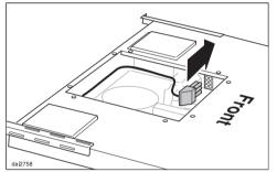
Plug the connector for the blower into the socket in the housing as shown.
