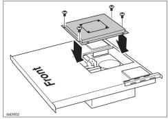
■ When finished, mount the previously removed cover on the front.
