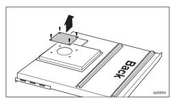
Remove the small cover on the rear of the ventilation system.
