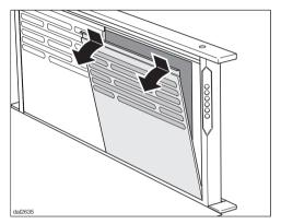
At the upper edge, push the grease filter down until you can pull it forward, then up and out.
