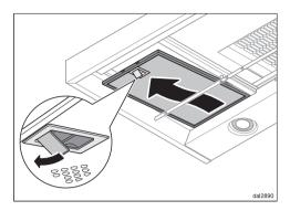
Open the grease filter lock, lower the grease filter slightly, unhook it at the back, and take it out.
