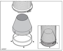
If you would like to reduce the environmental impact of your ventilation system by limiting the CFM output the Reducing Collar can be installed.
