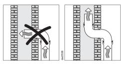
Never connect an exhaust hood to an active chimney, dryer vent, flue, or room venting ductwork. Seek professional advice before connecting an exhaust hood vent to an existing, inactive chimney or vent flue.
