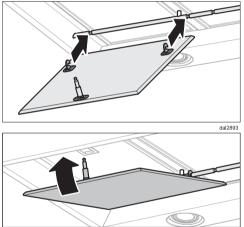
Hook the panels onto the support ledge, lift up the front and push them into the lock until they engage.
