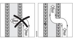
If the exhaust is ducted into an inactive flue, the air must be expelled parallel to the flow direction of the flue.
