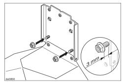
■ First loosely screw the two locking nuts onto the threaded bolts on retaining plate A.
