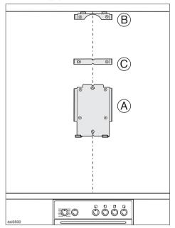
The ventilation system will be mounted to the wall through the use of retaining plates. Plate A is installed first, followed by plate B. Plate C should only be used if the distance between plate A and plate B is greater than 14  $^{3}/_{8}$ " (365 mm).
