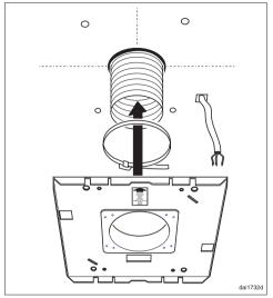
■ Secure the ducting to the mounting plate using a hose clip.
