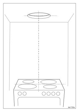
■ Cut a 7 ½" (190 mm) hole in the ceiling centered over the cooktop for the exhaust duct to pass through.
