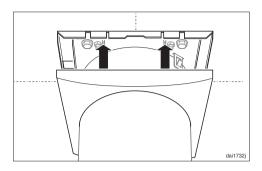
■ Finally, being careful not to scratch the chimney, push the cover plate upwards until the spring fixing clips click into place. If installed correctly, the cover should be secure and flush against the ceiling.
