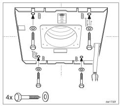
Screw the mounting plate through the ceiling and into the structural framing using 8 x 60 screws and washers. Once tight, make sure that the mounting plate can safely support the weight of the hood.
