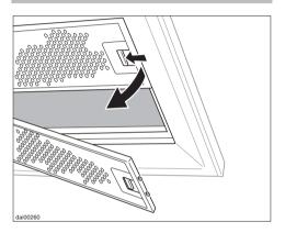
■ To remove the grease filters press the locking clips in towards the middle of the filter. Holding carefully, lower and remove the filter.
