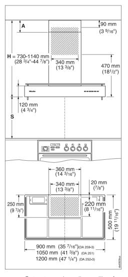
Cut out area in wall or ceiling for entrance of 6" (150 mm) ductwork or 5" (125 mm) ductwork with a reducing collar.
