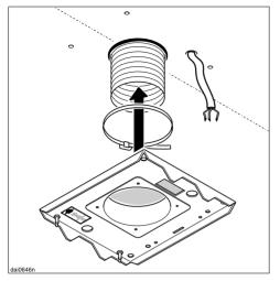
Secure the ducting to the mounting plate using a hose clip.
