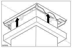
Finally, being careful not to scratch the chimney, push the cover plate up until the spring fixing clips click into place. If installed correctly, the cover should be secure and flush against the ceiling.
