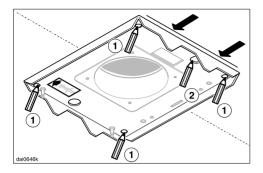
Hold the mounting plate up to the ceiling so that the orange arrow faces the front of the hood and aligns with the line drawn on the ceilling.
