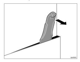
■ After removing the screws from the chimney, slide the lever between chimney and chimney extension and gently apply pressure to ease the chimney from its hooks.
