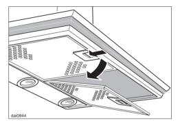
■ To remove the grease filters press the locking clips in towards the middle of the filter. Support grease filter so that it does not fall on to the cooktop.
