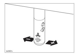
Use the joystick to select the desired time. Press it to the left for a shorter operating time, to the right for a longer operating time.
