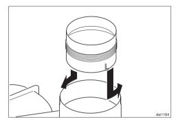
■ The reducing collar must be used in recirculation mode. Place the collars into the exhaust connections and turn left to lock them in place. Do not insert the non-return flaps.
