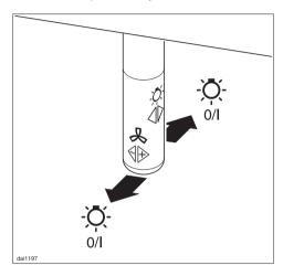
To turn the light on or off, press the joystick either once backwards or once forwards.
