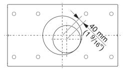
The exhaust connection is adjustable. This makes installation possible if the exhaust opening in the ceiling is not centered directly above the cooking surface. A maximum variance of 1 9/16" (40 mm) in each direction is possible.
