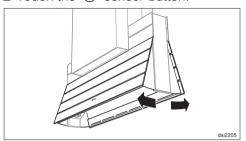
The fan switches on to level "2". The sensor buttons "①" and "2" light. The canopy now opens.
