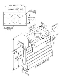
1) Feed-though for the duct work and the power cord
