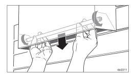
■ Rotate the fluorescent tube approx. 180° and downward to remove.
