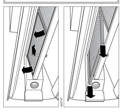
Press slightly upward on the grease filter handle to release it from the lower rail, pivot forward and lower it downward.
