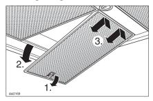
■ To remove the grease filters pull the locking clip forward. Lower the filter 45° unhook it at the rear and take it out. Support the grease filter so that it does not fall onto the cooktop.
