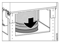
Place the exhaust ducting onto the exhaust socket.
