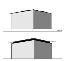
The **spacer frame** can be installed between the chimney and the ceiling. This creates a shadow which gives the illusion of a gap between the ceiling and the chimney. This is useful if the ceiling is not level or is uneven. The hood is aligned vertically with the spacers supplied. Visual irregularities between the chimney and the ceiling are then concealed by the shadow.
