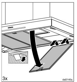
Remove the grease filters from the hood.
