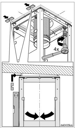
Align the installation frame and secure it with the screws.
