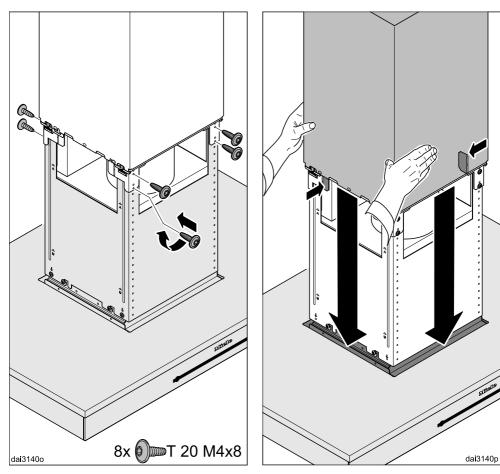
Raise the canopy to the desired height and secure it with the screws.  Hold the chimney securely, bend back the retaining tabs and carefully lower it.
