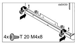
Secure the hood with the screws supplied.
