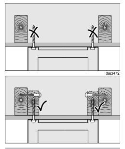
The hood must be attached to rigid structural framing that is supported in its entirety by the ceiling joists, or to the ceiling joists directly. Do not attach the plate directly to the ceiling with anchors, toggle bolts, etc.
