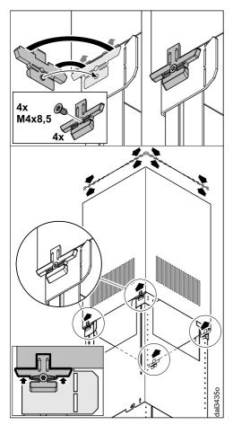
Fit the four telescopic chimney clamps. When the screws are tightened, the clamps spread out and push the telescopic expansion piece upwards.
