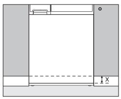
First of all you need to calculate measurement  $\mathbf{X}$ . This is the distance from the lower edge of the machine door to the lower edge of an adjacent kitchen unit door front.
