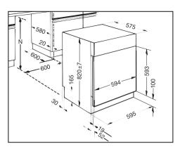
N = Niche height (820-930 mm) (illustration shows machine with lid removed)
