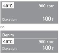
Press the Washing/Drying button repeatedly until **only** the Washing indicator light is lit up.
