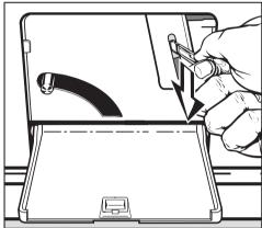
■ Insert a screwdriver into the notch, beside the lever, pull it down. The door will now open.
