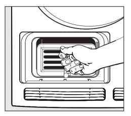
Pull the condenser unit out of its housing by the handle.
