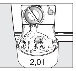
Unscrew the drain filter lid until water runs out.
