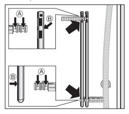
Secure the transit bars to the back of the washing machine. Make sure that holes
