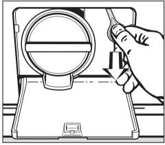
Pull the emergency release downwards (see illustration). The drum door will open.
