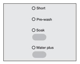
Press the appropriate additional option button. Press the top button repeatedly until the indicator light for the additional option you want comes on.
