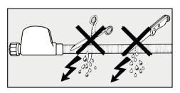
The protective sleeve of the hose must not be damaged or kinked.
