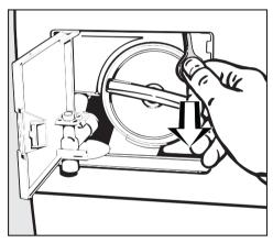
Pull the emergency door latch downwards (see illustration). The machine door will then open.
