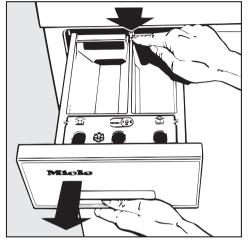
■ Press down the red release catch and at the same time pull the drawer right out of the machine.
