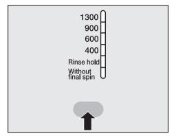
■ Press the "Spin" button enough times until the indicator light for the required final spin speed lights up.
