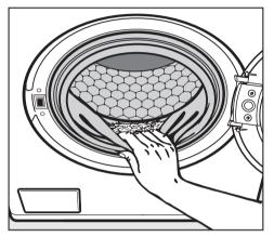
Check the folds in the door seal for any small articles, e.g. buttons which might be lodged there. Remove any fluff from drying from around the door seal.
