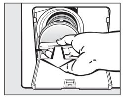
■ Unscrew the drain filter completely and then clean it thoroughly.
