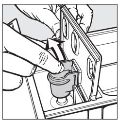
■ Remove the siphon tube from compartment 🕮 and rinse in warm water.
