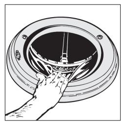
Check the folds in the door seal for any small articles such as buttons or nails which may be lodged there.
