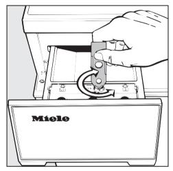
■ Turn the dial to the desired setting. Use the tool supplied with the machine. It is located behind the detergent drawer, on the left hand side (see Cleaning and Care).
