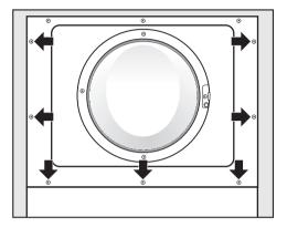
Screw the front panel to the machine door.
