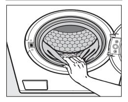
Check the folds in the door seal for any small articles, e.g. buttons, which might be lodged there.
