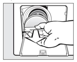
■ Unscrew the drain filter completely.
