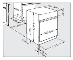
**N** = Niche height (820 - 930 mm) This machine is specially designed for installation under a continuous worktop run in a fitted kitchen.
