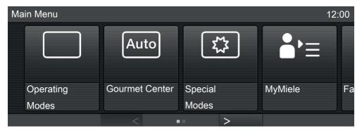
The top line shows what menu level you are currently in. Options within a menu are separated by a vertical line. If there is not enough space to show the whole path, additional options are indicated by ... I. The Time of Day, Alarm  $\overset{\sim}{\bigcirc}$  and Timer  $\overset{\sim}{\triangle}$  are shown in the top right-hand corner of the display.
