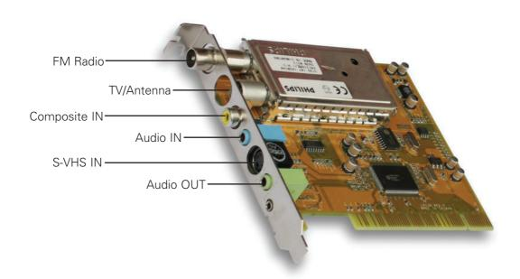
• TV/Antenna connection: This connector should be used for your analogue TV cable coming
