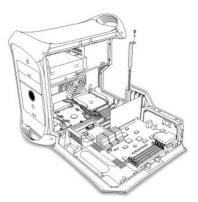
2. Align the connector end of the card with the PCI expansion slot and insert the card. Secure the card with the screw that you removed in the previous step.
