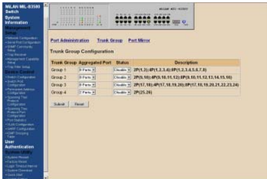
Figure 4-13. Trunk Group in Switch Port Configuration Menu
