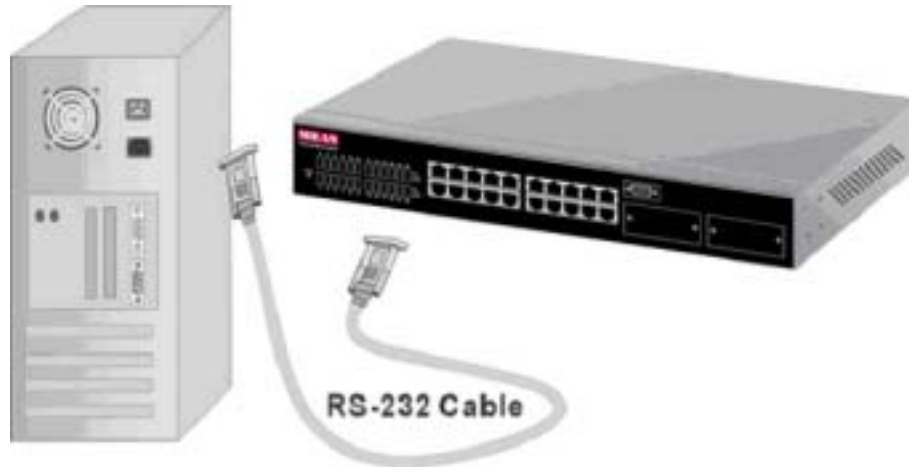
Figure 3-4. Connecting the MIL-S3580 to a Terminal via RS-232 Cable
