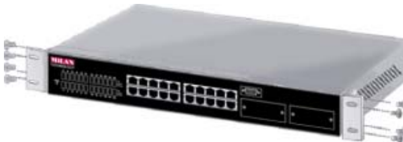
Figure 3-2. Attach mounting brackets with screws
