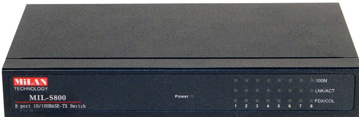
Figure 2. Front panel view of the MIL-S800
