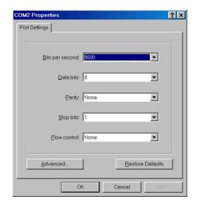
Figure 4-1. The settings of communication parameters
