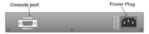
Figure 2-3. The Rear Panel of MIL-S8001TG switch
