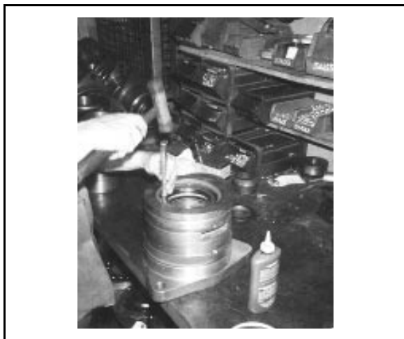
FIGURE 5 (MSSM0303AE) Installing Seals in Bearing Housing
