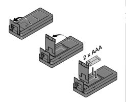
To ensure a reliable use, do not use zinc-carbon batteries.
