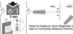
The minimum and maximum distance measured is displayed (min, max.). The last value measured is displayed in the main line.
