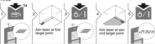
The result is shown in the main line and the measured value above.
