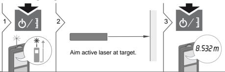
Target surfaces: Measuring errors can occur when measuring to colourless liquids. glass, styrofoam or semi-permeable surfaces or when aiming at high gloss surfaces. Against dark surfaces the measuring time increases.
