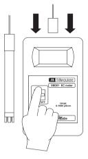
Adjust the calibration trimmer on the rear of the instrument with the supplied screwdriver until the display shows:
