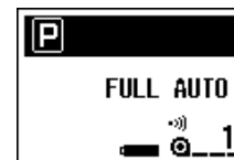
Example 2: Exposure-mode dial set to P , full-auto mode. Top part of display has turned black.
