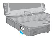
5 Lock the cover by sliding the latch to the left.
