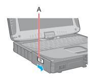
1 Unlock the cover by sliding the latch (A) to the right.
