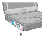
Slide the latch down, and then without releasing it, open the cover (B) as illustrated.
