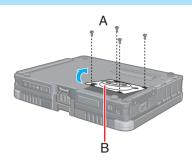
Turn the computer over and remove the screws (A), then remove the cover (B).
