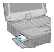
3 Simply slide the PC Card right-side-up until it snaps into place. Refer to the operating instructions of each card on how to insert the card.
