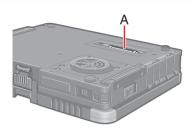
A port replicator is available as an option (CF-VEB181). This device eliminates the hassles of having you connect/disconnect the various cables when carrying your computer around and allows a variety of peripherals to be connected including a headphone or microphone, etc. The port replicator connects to the expansion bus connector (A) at the bottom of your computer.
