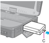
3 Pull the tab (C) on the hard disk drive and remove it from the computer.
