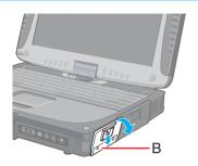
2 Slide the latch down, and then without releasing it, open the cover (B).
